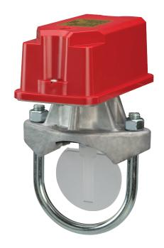
The new **WFDN Series** waterflow detectors from **Safe Signal** consists of a rugged, NEMA 4-rated enclosure that is more damage resistant than previous metal designs. The waterflow detector is designed for both indoor and outdoor use, with the widest available temperature range, from 32°F to 150°F. They are also approved for installation on the widest range of pipe schedules, sizes 2 in. through 4 in. are approved for installation on pipe schedules 7 through 40.
