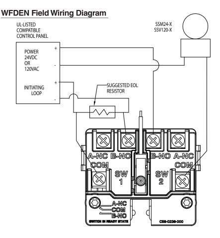
NOTE: COMMON AND B-NO CONNECTIONS WILL CLOSE WHEN VANE IS DEFLECTED, I.E., WHEN WATER IS FLOWING. DUAL SWITCHES PERMIT APPLICATIONS TO BE COMBINED ON A SINGLE DETECTOR.
